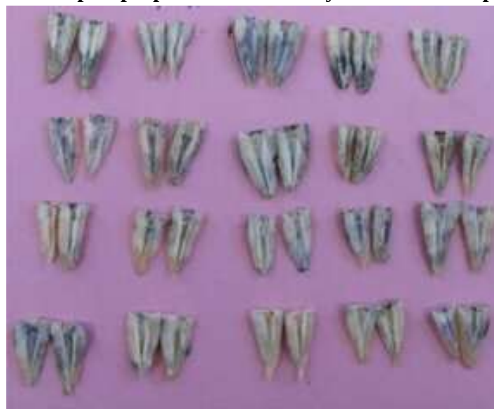
Figure 2. MTA samples prepared to study the extent of linear color penetration rate by a stereomicroscope
