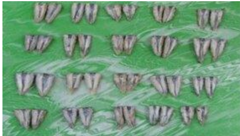
Figure 1. Resilon samples prepared for the study of linear color penetration rate
